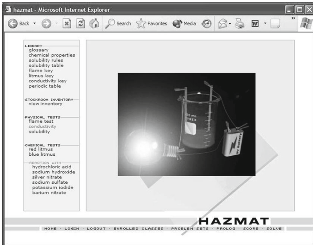
Fig. 27.2 HAZMAT. This screen shot of Hazmat shows the test items available (Library, Physical Tests, Chemical Tests) on the left side of the screen and a sample test result of a conductivity reaction in the center
